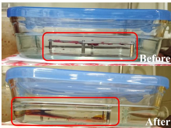
Fig. 28. Removal of solar cells by soaking in acetone solution in a glass case for about 10 days.
