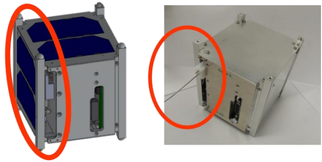
Fig. 20. Antenna deployment mechanism of ITF-1
