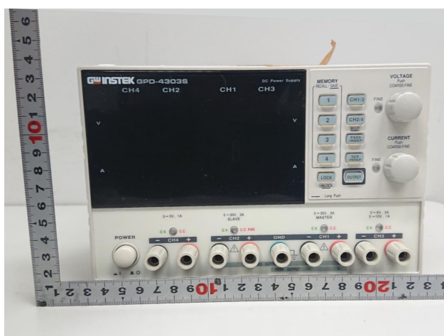
Figure 3.22 GPD-4303s front view.
